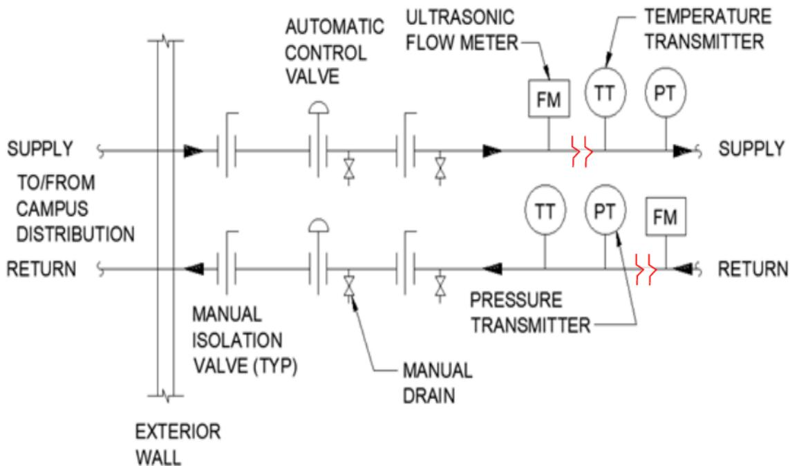
**CHILLED & HEATING WATER BUILDING CONNECTION DETAIL**
