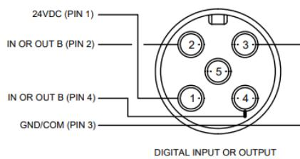
**4 M12 CONNECTOR PINOUT**
